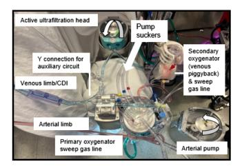
**Figure 5.** Picture of a Terumo CAPIOX FX-05 oxygenator with a neonatal/infant 3/16" arterial limb by <sup>1</sup>/<sub>4</sub>" venous limb circuit, modified with venous limb Y to allow for maximal secondary oxygenator flow (instead of standard venous line stopcock). For instructional purposes, the image depicts a secondary oxygenator replacing the hemoconcentrator for venous-assisted oxygenation (venous piggyback). Secondary oxygenator flow returns to top of CVR.
