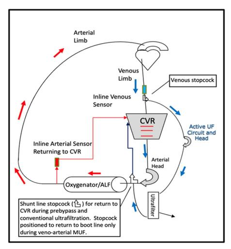
Figure 2. Schematic of CPB circuit with standard active ultrafiltration head incorporated. Blood can be sourced from the venous line for prebypass, conventional, and modified venoarterial ultrafiltration. This option exists on all circuit sizes.
